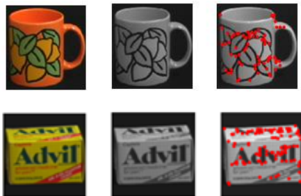
Fig. 6 Feature point extracted using FAST technique.
