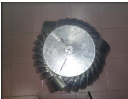
Fig. 19. Modified Turbine Ventilator
