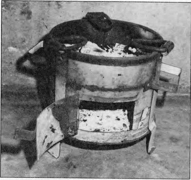
Fig. 1. A traditional metal charcoal jiko has an efficiency of 15–20%.
