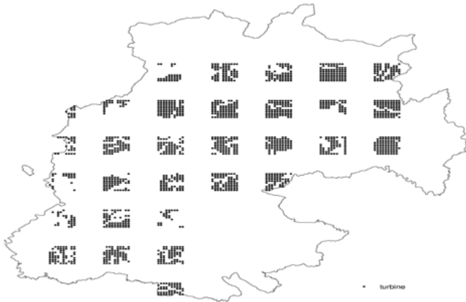
Figure 4. First hypothesis about plant areas location by considering allowed and high wind speed areas: in each area the allowed turbines.
