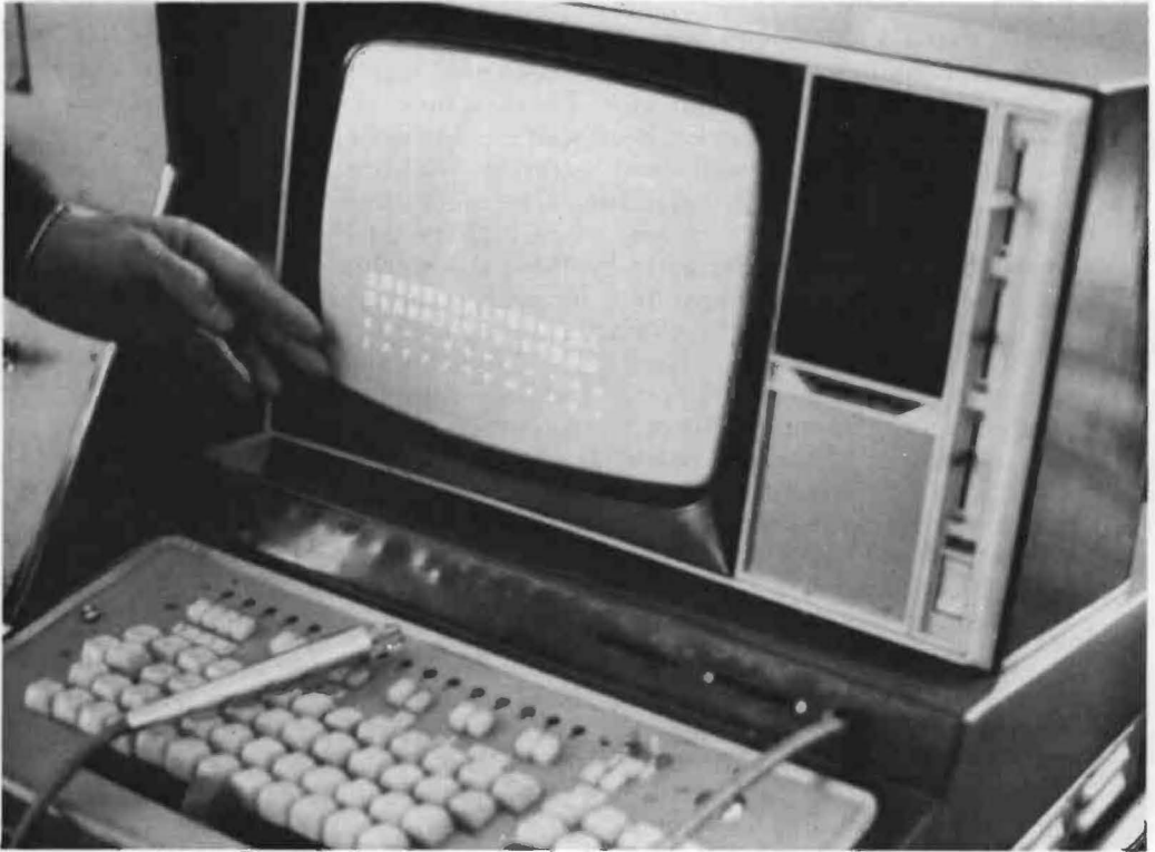
A CRT vector display with light pen (signowriter) is used for Chinese text input into the computer at BICT.
