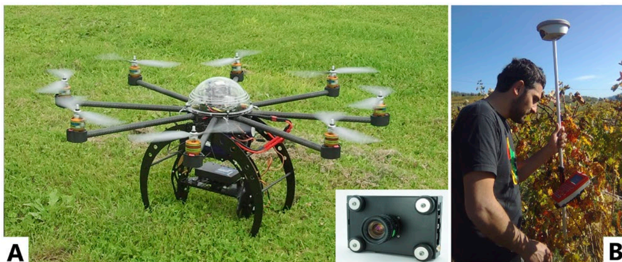
Figure 2. Instrumentation used in the study. A, Multirotor UAV platform (Mikrokopter, HiSystems GmbH, Moomerland, Germany), inset shows the multispectral camera (Tetracam ADC-Lite, Tetracam), B, Differential GPS (Leica GS09 GNSS, Leica Geosystems AG).
