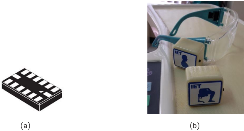
Figure 2. (a) accelerometer sensor model MMA7361L (b) head and upper arm sensor container
