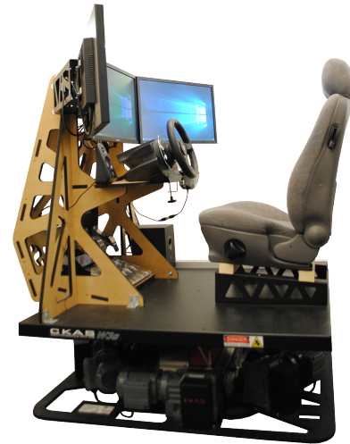
Figure 1: Cockpit mockup on the motion platform.
