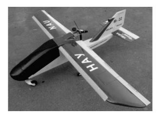
**Technical Characteristics:** Wingspan – 2.5 m; Weight of special purpose load – up to 8 kg; Launch weight – up to 18 kg; Top speed – 120 km/h; Engine power – 2.7 kW; High flight altitude – up to 2000 m; Method of launch and landing – as an aircraft; Deployment time in the working position – 0.5 h.
