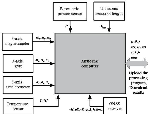
Fig. 1 Structural scheme of integrated navigation system
