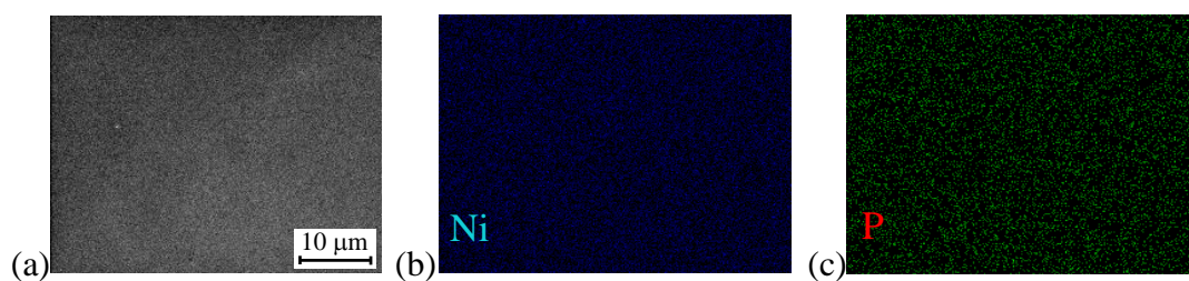
Fig. 5.11 Elemental mapping analysis of work surface after scanning polishing for 60 min: (a) SEM image, and distributions of (b) P and (c) Ni
