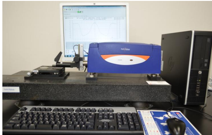
Fig. 2.5 Taylor Hobson Form Talysurf Intra profilometer
