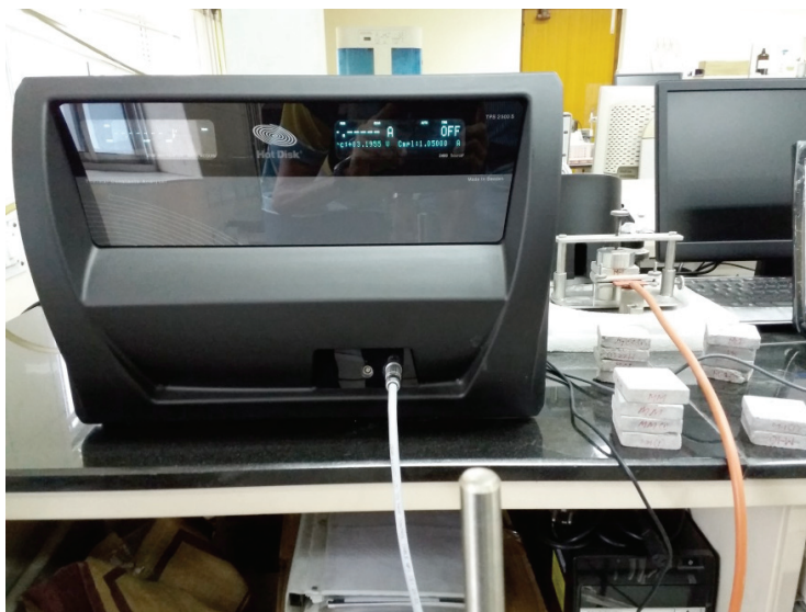
Fig.1 Thermal Conductivity Test Set up
