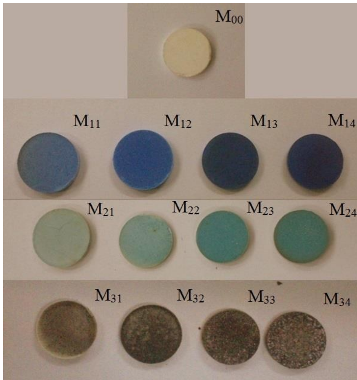
Figure 6: Digital images for the pellets of pure and transition metal ions conjugated mullite composites after sintering at 1300°C.
