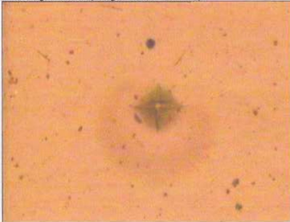
FIGURE A Micrograph of indentations – GL 092 – 1N 500x magnification (image width 0.0625mm)
