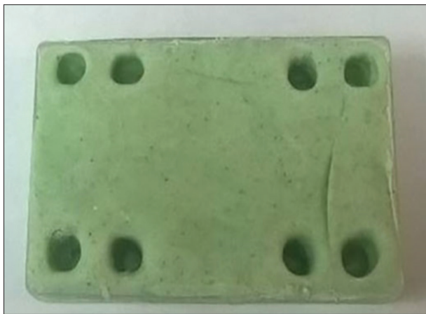
Figure 2: A rectangular acrylic block with eight holes in each block to support the teeth
