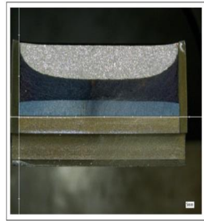
Figure 8b The crack propagation in the SENT specimen
