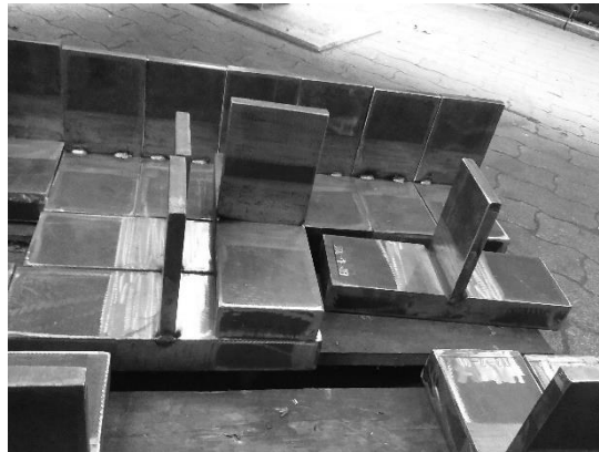
Fig. 1 Tack welded T-joints before welding.
