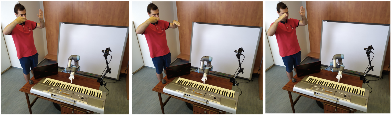
Fig. 6. The robot gets a task to reach the position of “so” (left figure), then presses the not (middle figure), and repositions himself to “re” (right figure).
