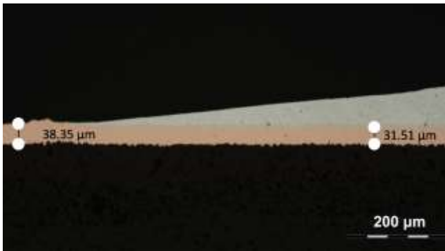
Fig. 6. The difference of the copper clad thickness
