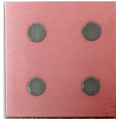
Fig. 2. PCB sample before the soldering
