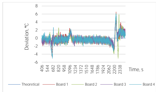
Fig. 6. Deviation of theoretical programmed and measured temperatures.
