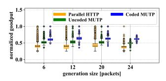
**FIGURE 13.** Normalized goodput of downloading 1-2MB chunks with generation size  $g \in \{12, 20, 24\}$  over one 1,792 KB/s and three 896 KB/s connections with window size w=240.
