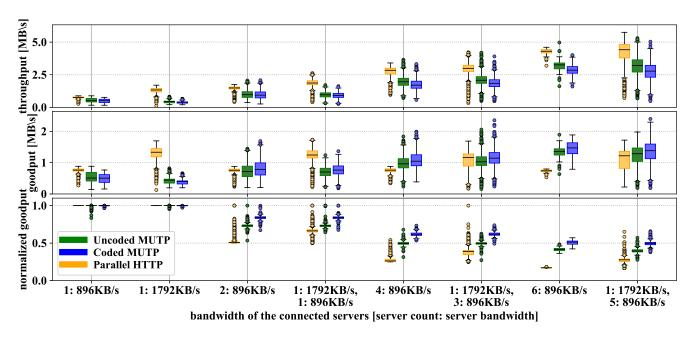
FIGURE 11. Grouped boxplot representation of downloading 1-2MB data from  $N \in \{1, 2, 4, 6\}$  servers with 896 KB/s and 1,792 KB/s upload bandwidth with window size w = 240 and generation size g = 24.
