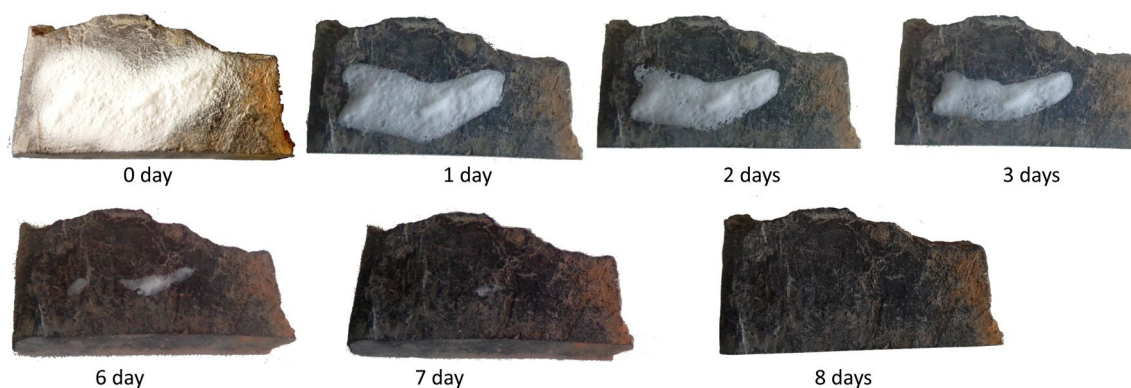
Fig. 1 The sublimation of a 1-mm-thick cyclododecane coating at an ambient temperature from a porous pottery fragment
