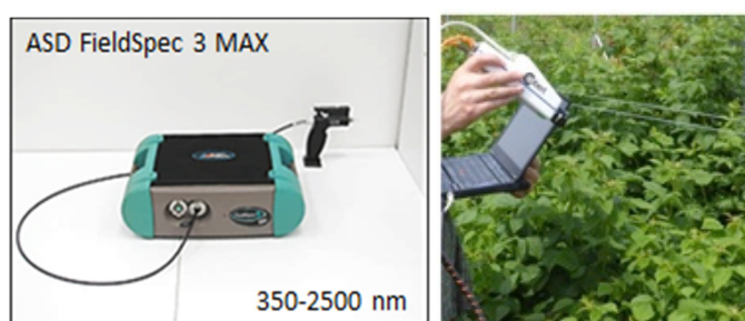
Fig. 2: ASD FieldSpec 3 MAX (350-2500 nm) and Cuber UHD185 (400-1000 nm)
