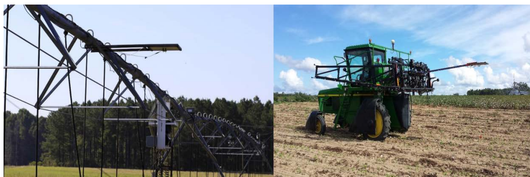
Figure 1. GPS antennas mounted on lateral VRI (left) and on a high-boy sprayer (right) during 2013 and 2014, respectively.
