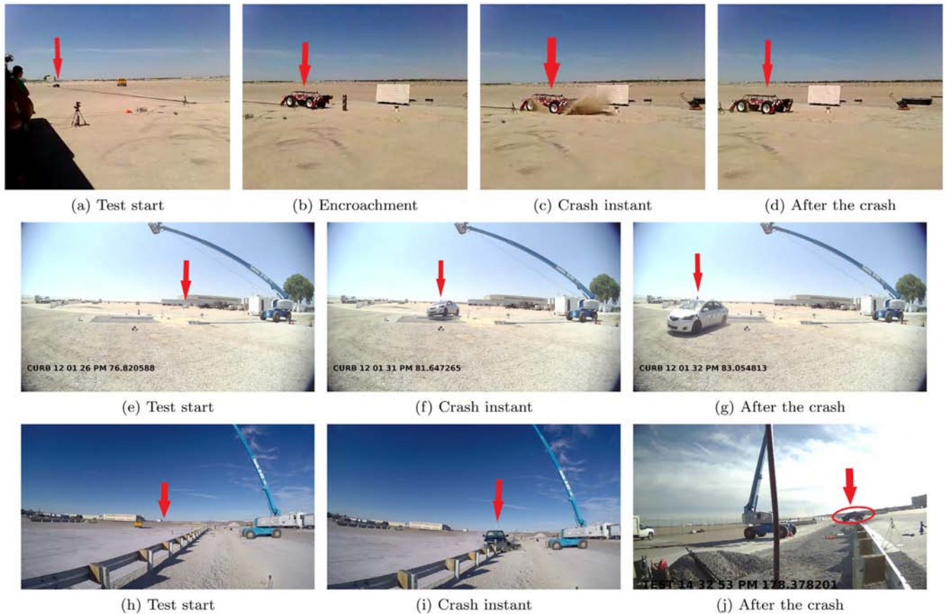
Fig. 6. Snapshots of different stages of crash tests: (a–d) Bogie, (e–g) Sedan, and (h–j) Pickup.
