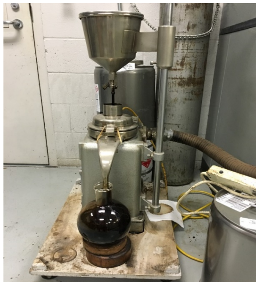
Figure 3-4. Micro-centrifugation of the solution after extraction.
