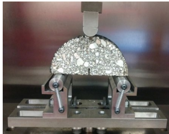
Figure 3-10. SCB testing set-up.
