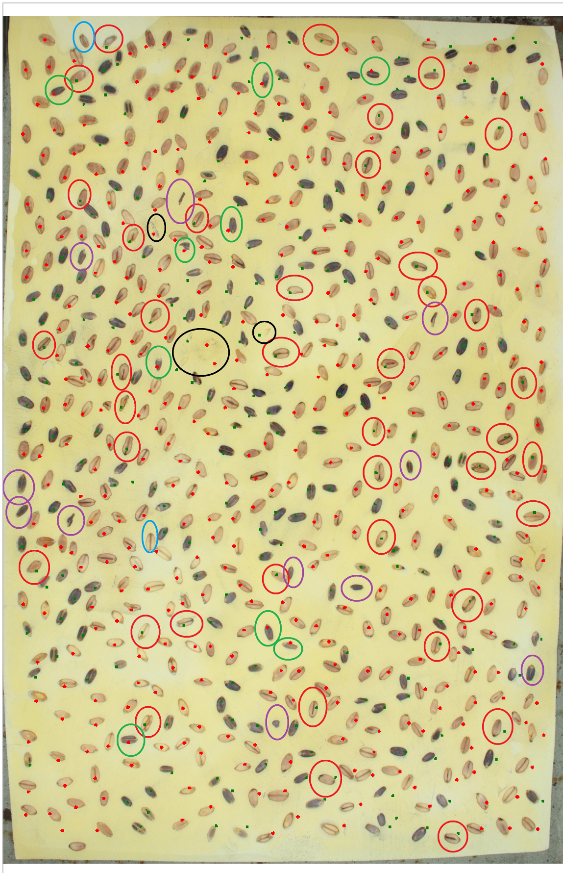
Figure 6. Photograph of one test sample (Pair 5, 25% conventional) in which a visual check of PLSDA (preprocess of SNV and first derivative) classified kernels was performed by embedding kernels in a polymer clay, heat curing the slab, sanding the slab's surface to expose kernel endosperm and staining with an iodine solution. Red and green dots correspond to the centroidal positions of classified respective waxy and conventional kernels in the hyperspectral image that have been superimposed on the photograph. Coloured circles are defined as follows: red = visually identified as waxy but classified as conventional; green = visually identified as conventional but classified as waxy; black = kernel(s) lost during sanding.
