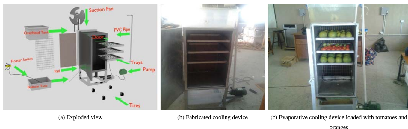
Figure 2 Exploded view of the evaporative cooling system and fabricated cooling system
