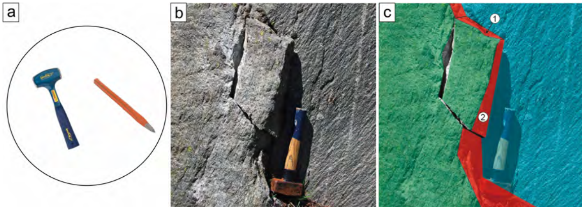
Figure 8.3: (a) Example of a chisel and shorthanded sledgehammer. (b) Picture of a surface sample along the Montenvers transect (sample MBMV7). (c) Schematic of the sample surface showing the surface of interest (in green), the free surfaces (1) horizontal and (2) vertical (in red) and the unwanted surface (in blue).
