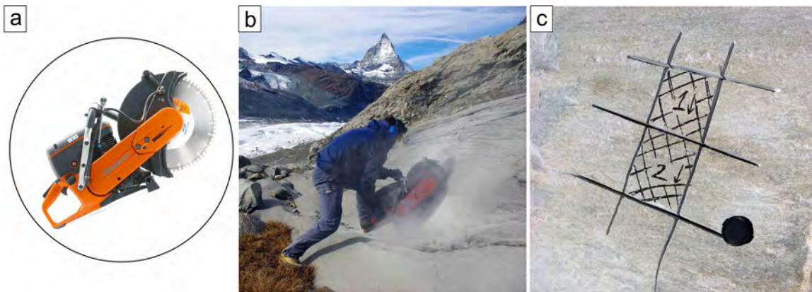
Figure 8.5: (a) Example of a fuel powered power cutter mounted with diamond blades (Husqvarna power cutter K760 model in the present case). (b) Sebastian Vivero sampling a polished bedrock surface on the side of the Gornergletscher for Joanne Elkadis PhD project. (c) Picture of the resulting cut in the bedrock, providing two blocks of sample (arrow showing the direction of the steepest descent in order to orientate the sample once in the lab).
