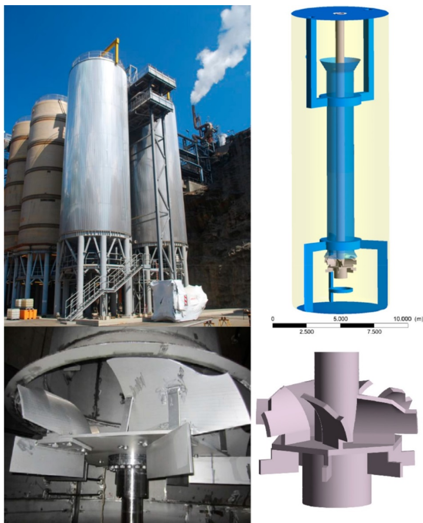
Figure 1. Industrial scale OKTOP®9000 reactor (left) and CAD geometry for large-scale reactor and impeller (right). Adapted with permission from Outotec Oyj
