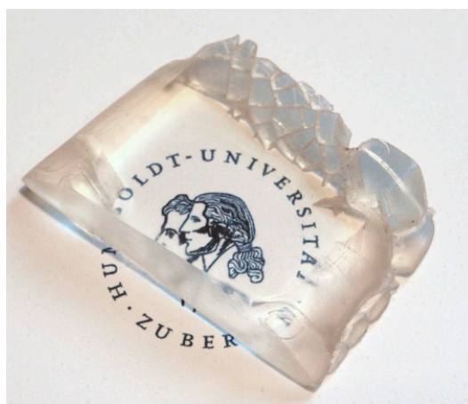
Figure 19. Photograph of a representative composite sample with MgF 2 (10 wt %) in PolyHEMA. Reproduced from Reference [62] with the permission of the Royal Chemical Society.
