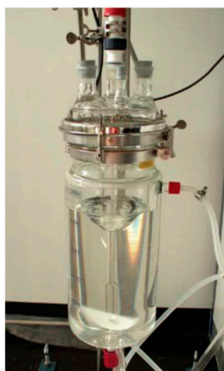
Figure 5. \text{MgF}_2 sol stabilized by \text{Al}(\text{O}^i\text{Pr})_3 after 2 days of fluorination prepared in a 10 L reactor. Reproduced from Reference [37] with the permission of the Royal Chemical Society.
