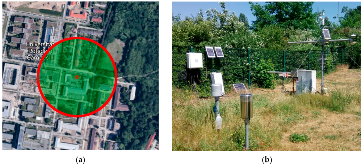
Figure 4. (a) Campus of Potsdam University, red point is where CRNS probes were installed and the red circle is the footprint. (b) Picture of the installation.
