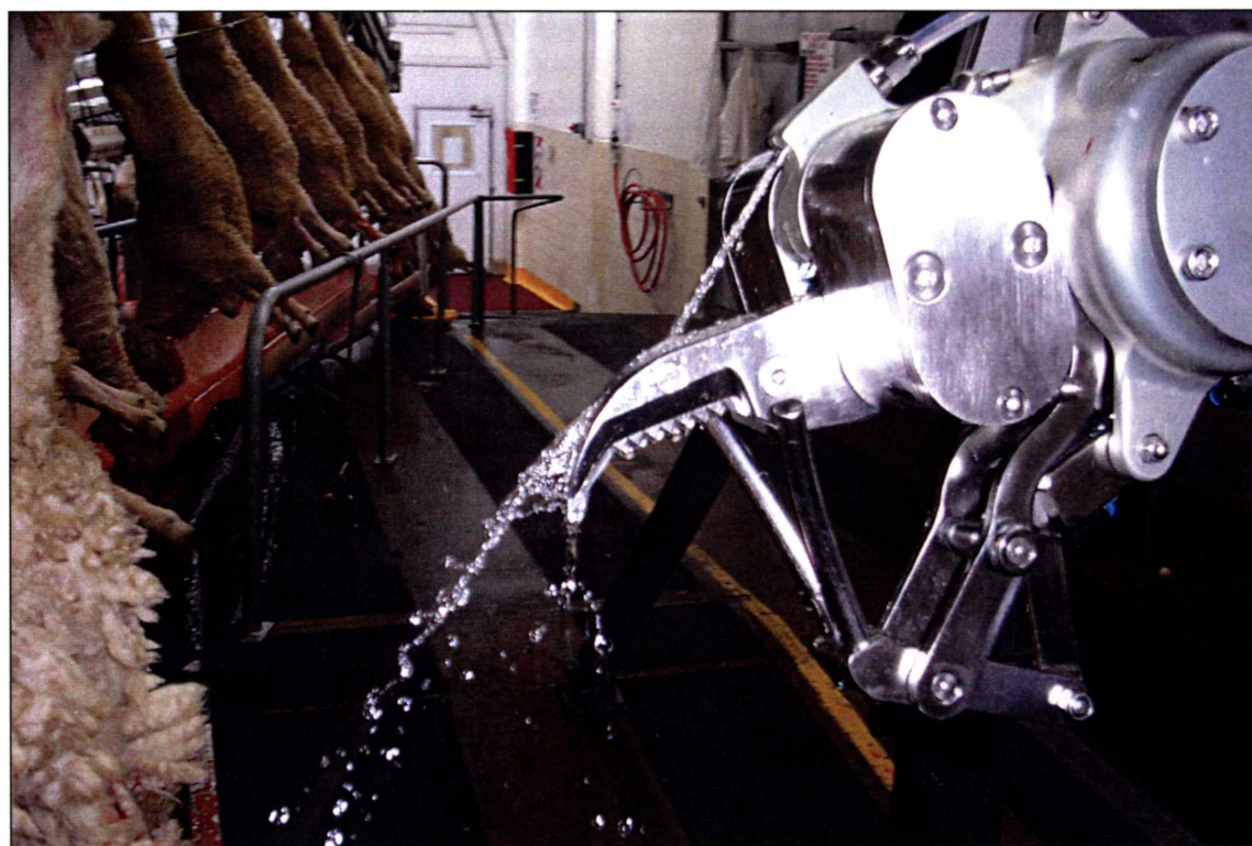
FIGURE 3.5 Sterilisation of the blades using an integrated spray nozzle.
