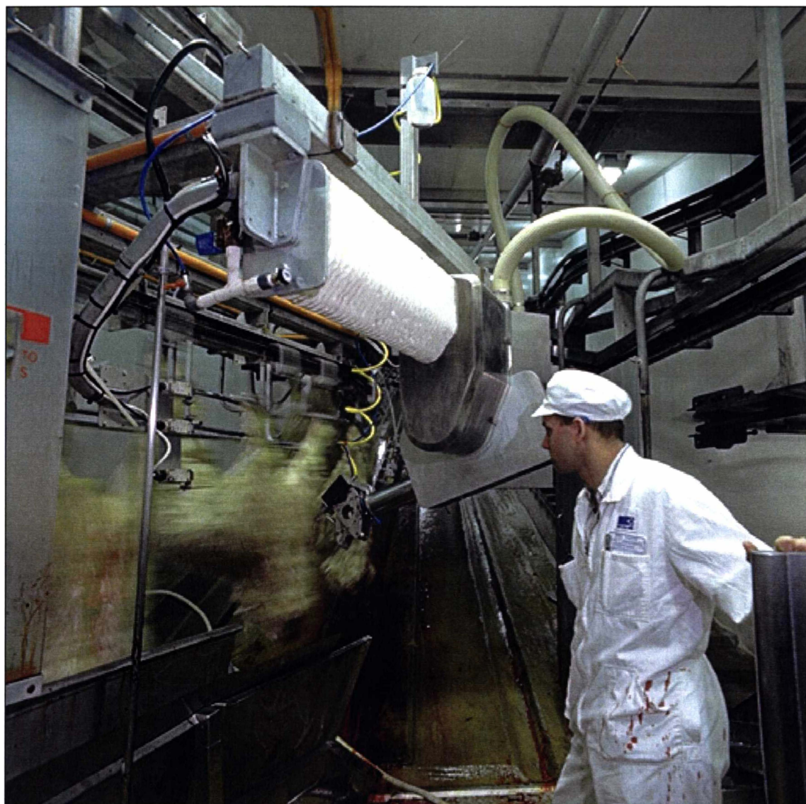
FIGURE 3.12 The IRL8L Y-cutting robot in action at Alliance Smithfield.
