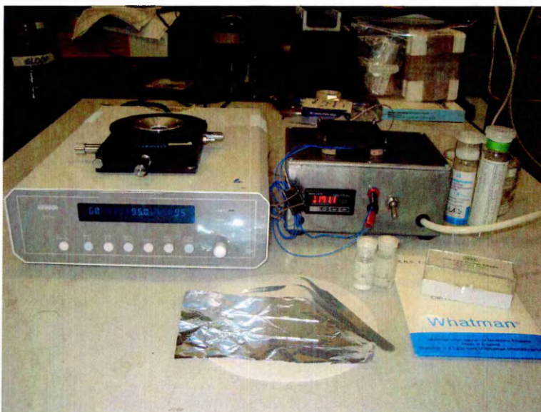
Figure 4.2 Photograph showing the two hot-stages used to grow HB oligomer spherulites from the melt in this project. Left hand side is a Linkam hotstage, right a thermal hotstage constructed for this project.
