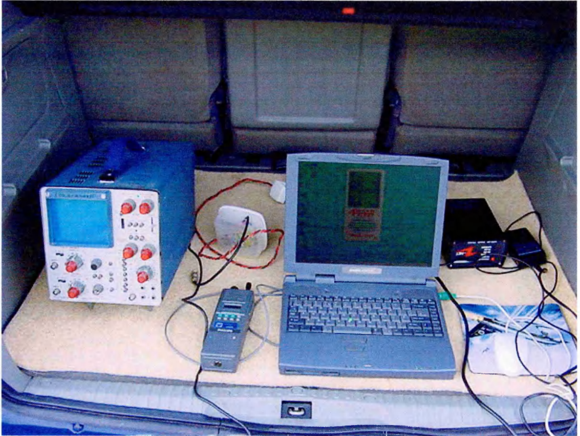
Figure 38 Nimbus Mk1 PLM Receiver Set Up in Nimbus vehicle
