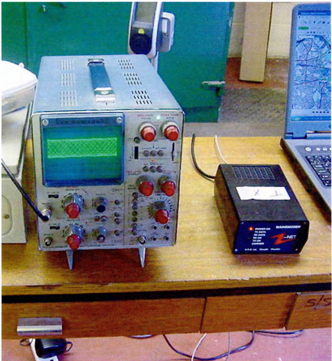
Figure 40 DM 64 Oscilloscope with Transmit signal from the Nimbus Mk1 PLM
