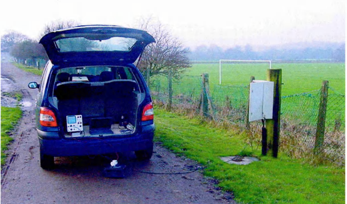
Figure 39 Vehicle with Nimbus Mk1 test system connected to HAP
