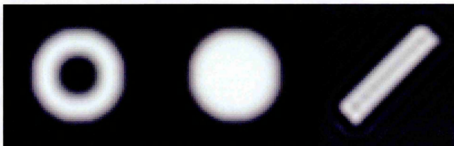
Fig. 3.4b The radius of gyration R_{gyr} for three different images demonstrates its strengths and weaknesses. R_{gyr} measures 16.0 for the left hand ring, 14.5 for the central disc and 14.5 for the rod. It successfully distinguishes the disc from the ring, which have identical maximum radii. However, although their shapes are totally different, it cannot distinguish the rod from the disc, which have identical R_{gyr} values.
