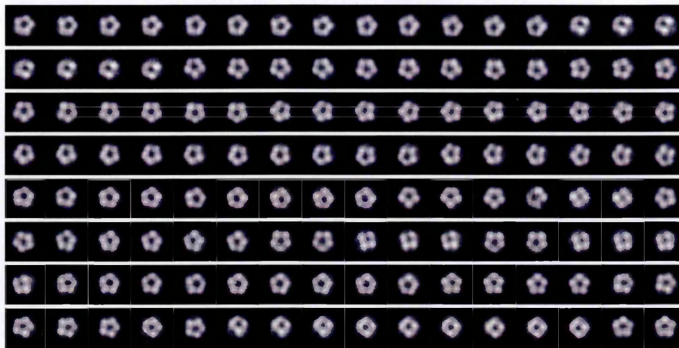
Fig. 3.7 A set of candidate images selected by this algorithm from part of a micrograph image of KHMT particles. The program computes a linear array of boxes. For display purposes the array is shown here arranged in rows such that the first particle in the array is top left and the last is bottom right. There are several sets of overlapping windows for each particle which are clearly not grouped contiguously. Since in the program the window moves across the digitized image from column to column for each row, the windows are ordered first according to their column, then row. When there are several different particles in a single row in the image, then only portions of a candidate cluster are arranged in contiguous order. For example, in row 6, images in positions 9-11 are overlapping windows of the same images as those in positions 14-16 (and position 1 in row 7).
