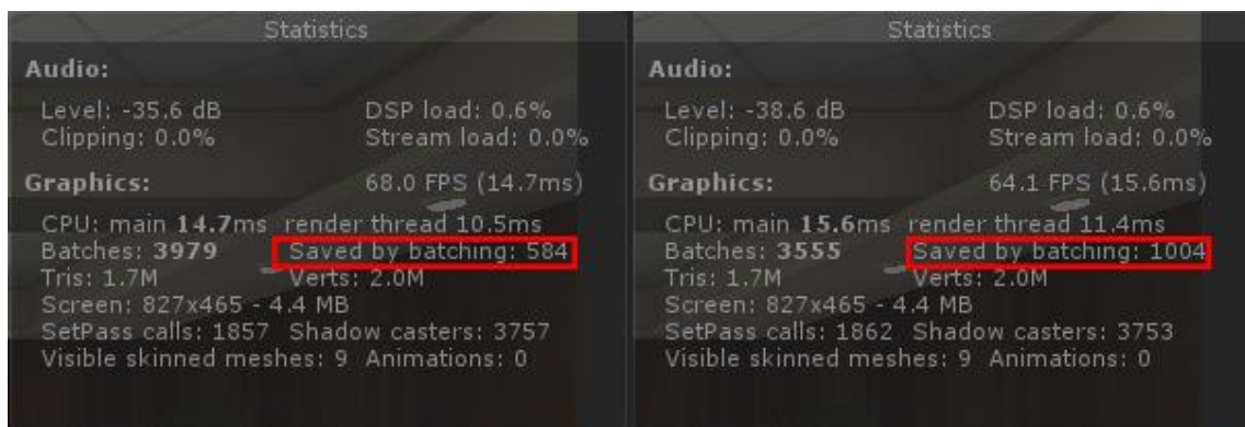
Figure 30: GPU instancing disabled (left) and GPU instancing enabled (right)
