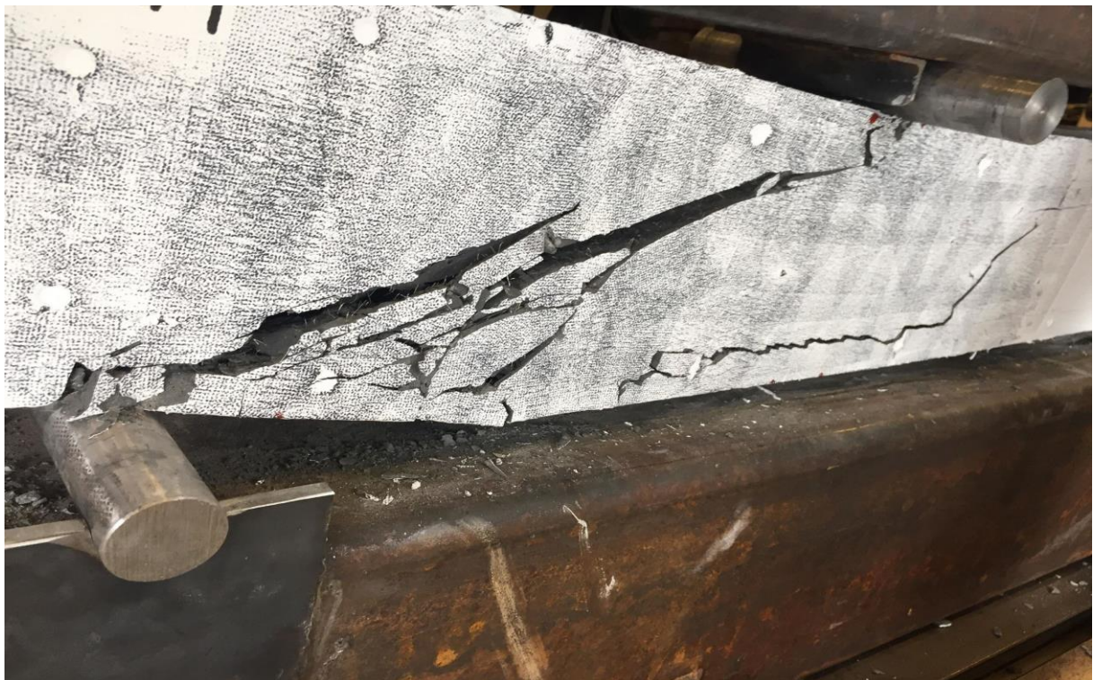
Figure 7-7 Shear crack pattern of the beam- G1- 0.5% fibre
