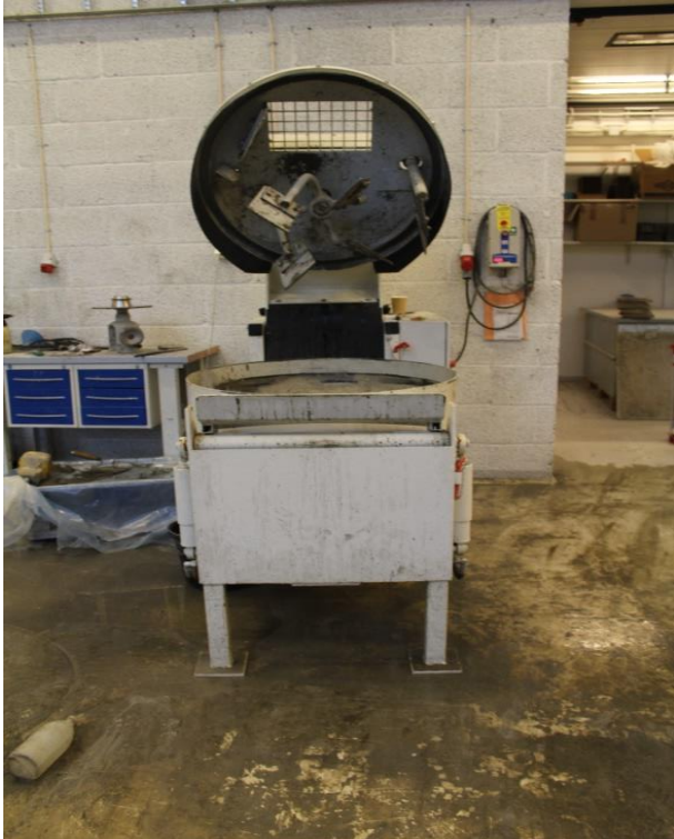
Figure 5-2 The used mixer in our experiments- Zyklos
