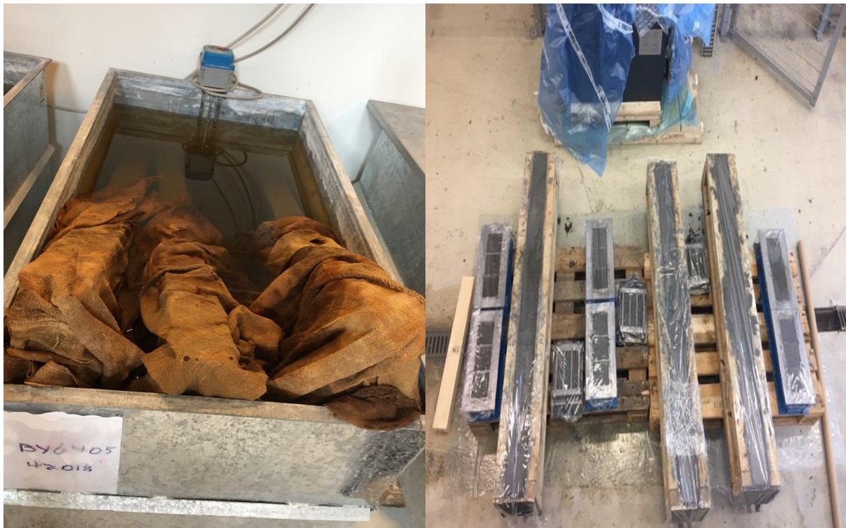
Figure 6-4 The cast specimens
