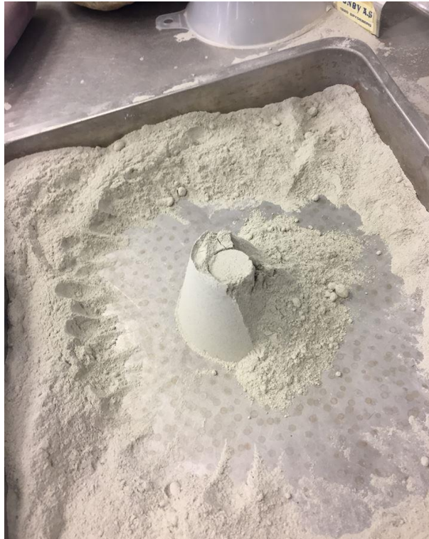
Figure 6-2 Saturated Surface Dry of our work in the lab
