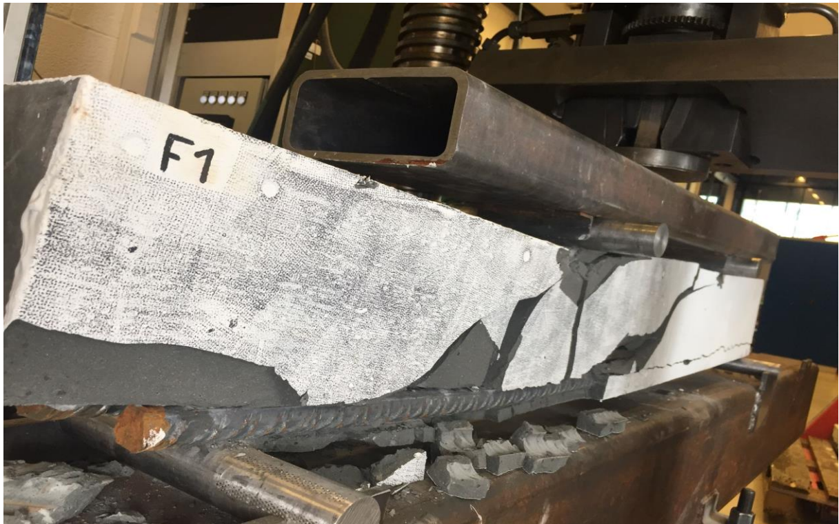
Figure 7-6 Shear crack pattern of the beam- F1- 0% fibre
