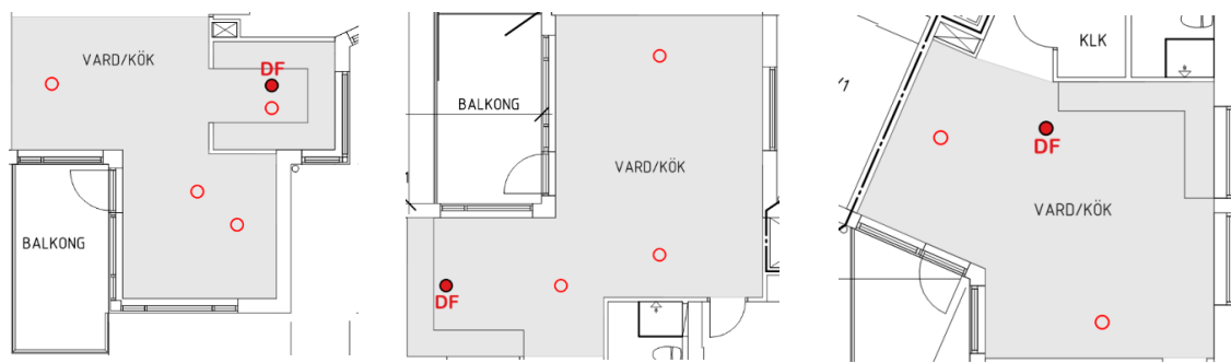
Figure 6. Examples of combined kitchens and living rooms that result in complex floor layouts. Acceptable positions for the evaluation of single-point DF are indicated with circles. Positions with the lowest calculated single-point DF are shown by dots.
