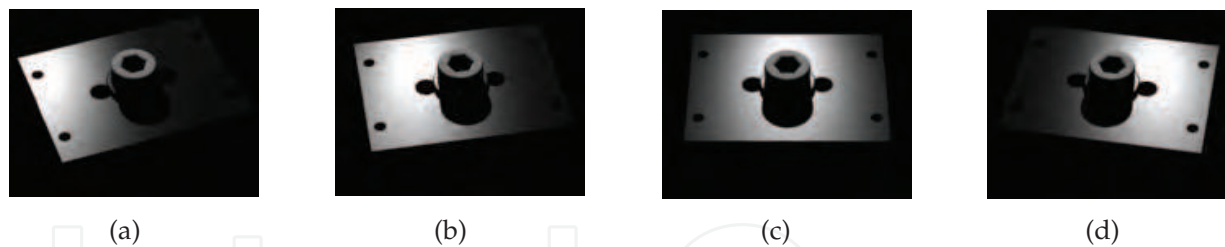
Fig. 5. Series of synthetic images of an assembly under fixed illumination and moving camera. The Phong reflection model was used with different parameters for the parts of the assembly.
