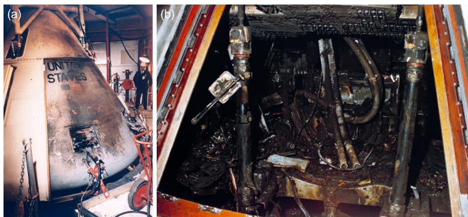
Figure 1.1.1 Apollo 1 fire: (a) blackened command module and (b) charred remains of the Apollo 1 cabin interior.
