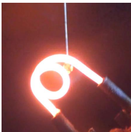
Figure 2.2.1 Hot surface ignition for a droplet with FeCr wire.
