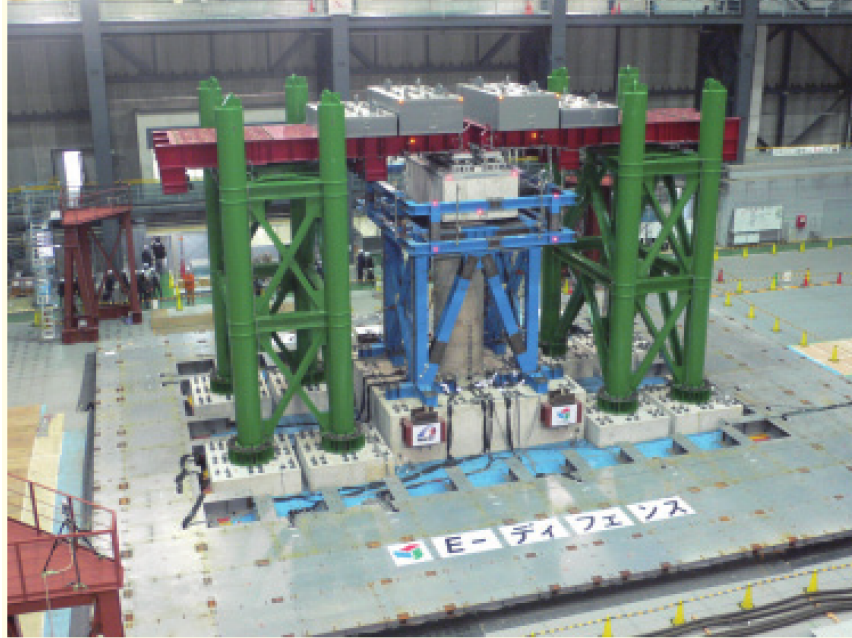
Figure 2-1: C1-1 Experiment setup on E-Defense shake table [1]
