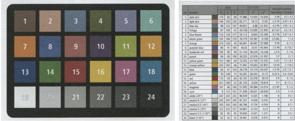
Figure 2.3: (left) X-Rite ColorChecker Color Reproduction Chart. (right) Colorimetric values for each patch in the charts.[63]
