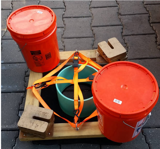
Figure 4: Surface infiltration test apparatus
