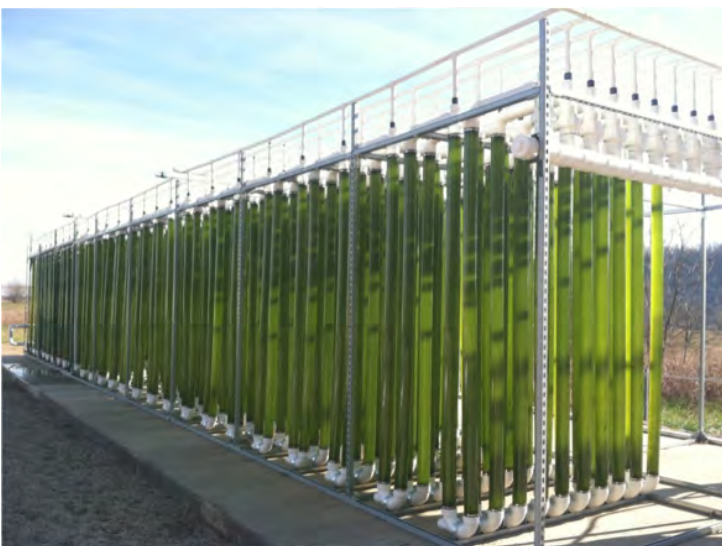
Figure 8. Side view of completed photobioreactor at East Bend Station comprised of 500 3.5" tubes for a total volume of 18,000 liters.
