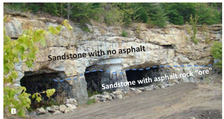
Figure 10. Views of various ways of extraction of asphalt rock in Kentucky (A)strip mining and (B)room and pillar accessed through tunnels or adits. View A is an early 1900s aerial view of the communities of Kyrock, Ridgedale and Woodside (extant today) along the Nolin River in Edmonson County where strip mining or quarrying occurred. View B is a 2007 photo by author near Sweeden, KY in Edmonson County – Indian Creek Quarry (historic image in (A) courtesy Kentucky Museum Library – Western Kentucky University, Bowling Green).
