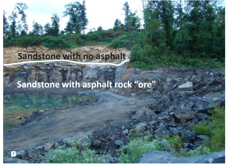
Figure 9. Asphalt rock or tar sand in Edmonson County: A) close up view of typical flow of hydrocarbon out of rock - for scale note that hammer head is 7 inches long (18 cm) B) view of reopened quarry with rock devoid of bitumen overlying asphalt productive zone (both photos by author in 2010).
