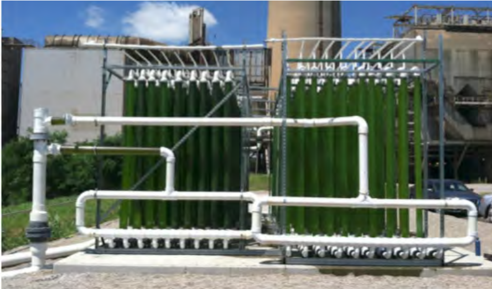
Figure 7. Feed end of photobioreactor at East Bend Station showing an operational comparison of 5" tubes (left) vs. 3.5" tubes (right).
