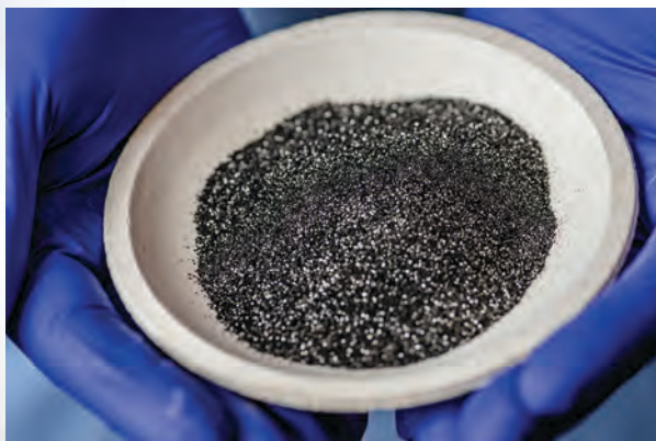
A sample of Drelich's copper-vermiculite material. It represents a tremendous opportunity to battle bacteria and prevent infections. Early tests look to be extremely promising.
