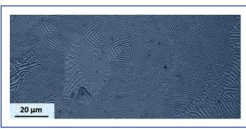
A Zn-3Mn eutectic alloy, showing Mg2Zn11 in a spiral pattern within the hcp Mg matrix. Optical micrograph by Ehsan Mostaed, MSE postdoctoral assistant.
