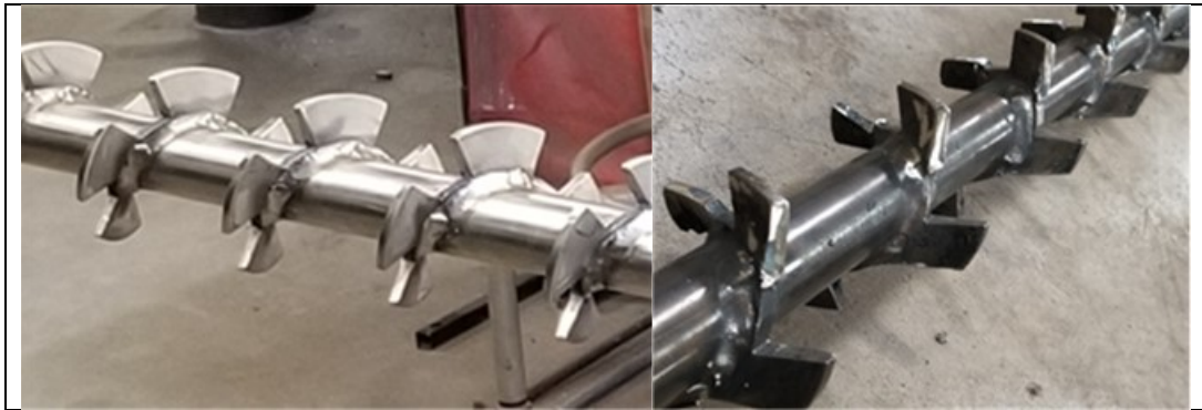
Figure 7.1. Shaft before (left) and after (right) modifications.
