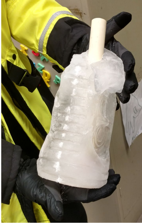
Figure 3.32 Ice cylinder with frozen-in PVC for ice borehole experiment.
