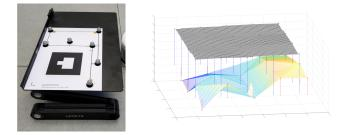
Fig. 7: Combined FM-Vicon Marker (left) and qualitative evaluation (right) of various measurements of the FM-Vicon marker on the plane floor of the *CITrack* laboratory for a single camera. Black surface is measured by Vicon while the other is measured by *ArUco*.
