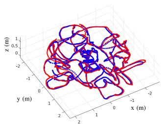
Fig. 8: Calibration walk as tracked by Vicon (blue) and the final calibrated *CITrack* in an operative hight between 0 m and  $\sim$ 1 m wrt. the floor. The two point clouds do overlap sufficiently well with little disturbances at the *CITrack* boarders (e.g. (x,y)=(1,-3) m).
